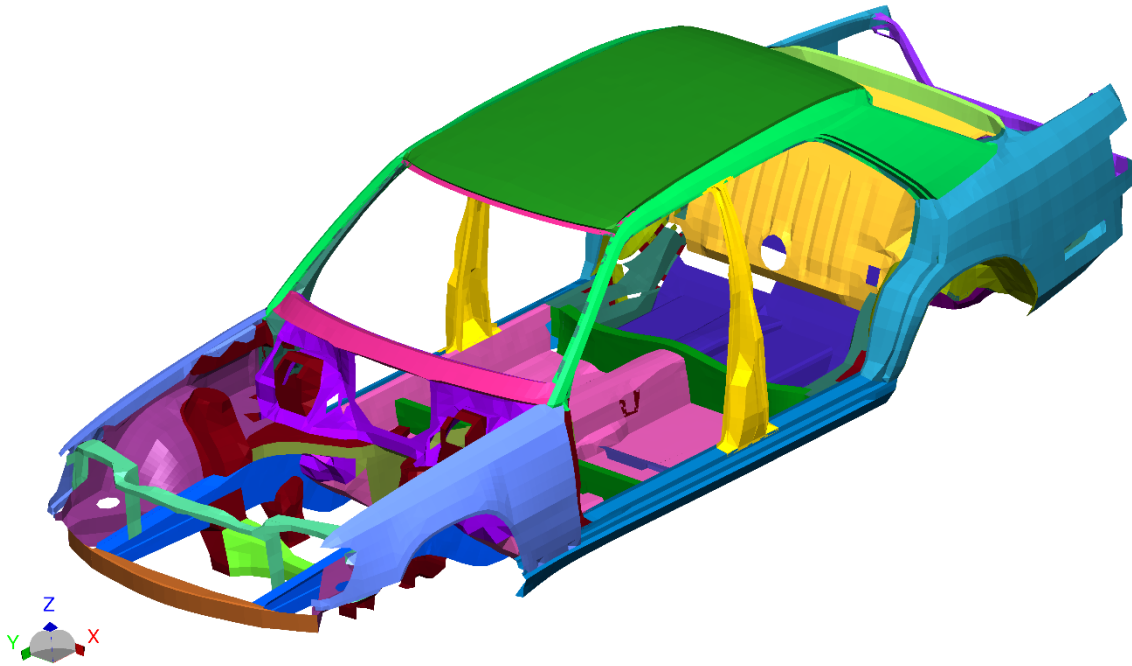
Fig. 1: Body-in-white finite element model
