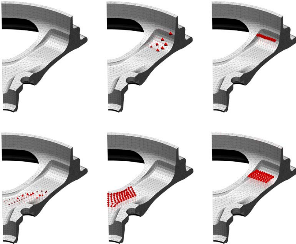
Figure 10: Original shape and 5 shape basis vectors for the shape modification of the “old” wheel geometry.
